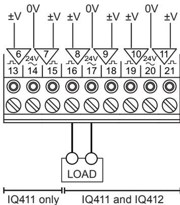
Each output provides an independent 24 Vac feed for driving 24 Vac loads, such as thermoelectric (thermic) actuators, and raise lower actuators, (e.g. the Trend range of thermic actuators).
