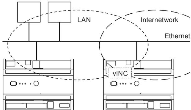
In addition, the IQ41x has the ability to join an internetnetwork using its virtual INC (see 'Networking' on page 4 for further details).
