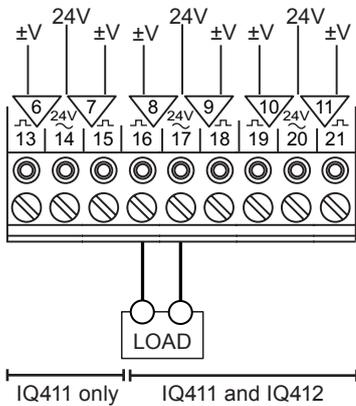
**IQ41x/230:** Switches 24 Vac (synthesised), 300 mA maximum for a channel, 300 mA maximum shared between all (4 or 6) channels. Terminals and example wiring:
