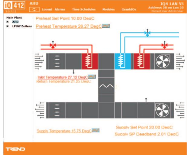
General and Item alarms can be sent either to a designated Trend LAN address, to an IP address, or as an email. Alternatively, certain Item alarms (sensor, digital input, digital driver readback, and plot), can be sent to a BACnet device.
