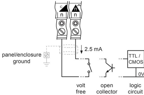
The volt free contact has a nominal wetting current of 2.5 mA. The input is ON when the contact is closed. There is no polarity.
