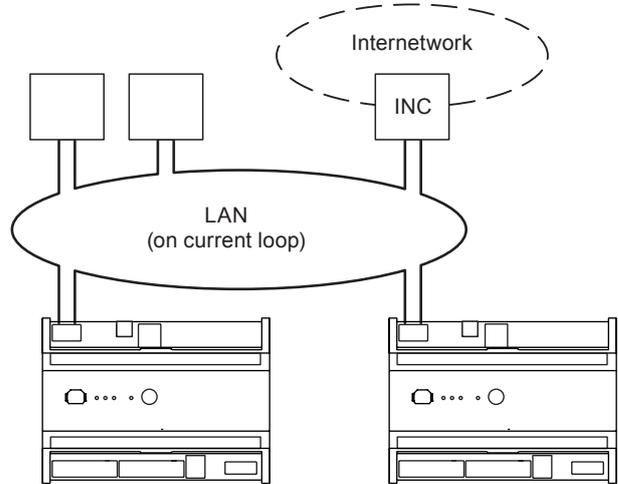
*Note: In this configuration IQ41x cannot join a Trend LAN on Ethernet. However, access by IP is still possible.*
