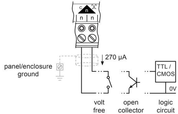
The volt free contact has a nominal wetting current of 270 µA. The input is ON when the contact is closed.
