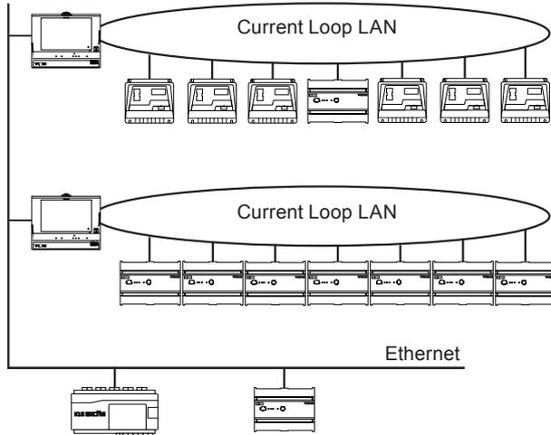
The diagram above shows IQ41x/LAN replacing/extending an IQ21x system on the Trend current loop LANs, and an IQ41x connected to a Trend Ethernet LAN.
