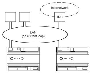
Note: In this configuration IQ41x cannot join a Trend LAN on Ethernet. However, access by IP is still possible.
