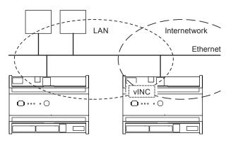
In addition, the IQ41x has the ability to join an internetwork using its virtual INC (see 'Networking' on page 4 for further details).
