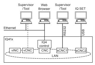
**Default CNC Addressing**: The IQ41x device (outstation) address is factory-set (in the Address module) as follows:
