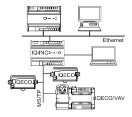
Note: There can only be one IQ4NC on the MS/TP trunk. The LAN number is read-only in the IQECO and is set up when it is installed by the IQ4NC (default LAN 9).
