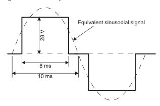
For time proportioning drivers (in power managed mode) a 'soft start' of the above waveform is implemented to allow for the large inrush currents of thermic actuators.
