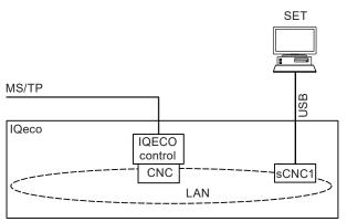
**Default CNC Addressing:** The IQECO's Trend device address is set up in the factory on a rolling basis in the range 11 to 119. So in a batch of IQECOs, each will have a different device address (printed on the unit's label along with its unique serial number).
