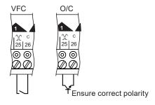
The volt free contact has a nominal wetting current of 270  $\mu$ A. The input is ON when the contact is closed. There is no polarity.
