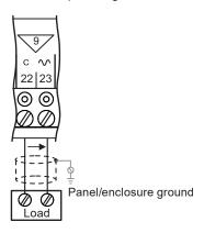
Use 2-wire twisted screened cable for wiring the outputs, with the screen connected to the panel/enclosure ground and unterminated at far end. Connect the return to the C terminal (e.g. 22 C) not to an input common.
